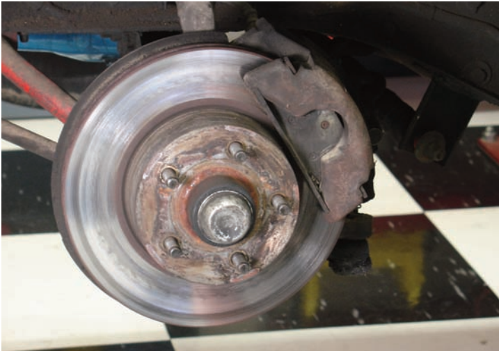
In 1967 Ford introduced disc brakes with four piston calipers, but because of problems the disc brake system was changed to dual piston calipers in 1968 as shown here. This is the original brake system that was delivered by the factory.
