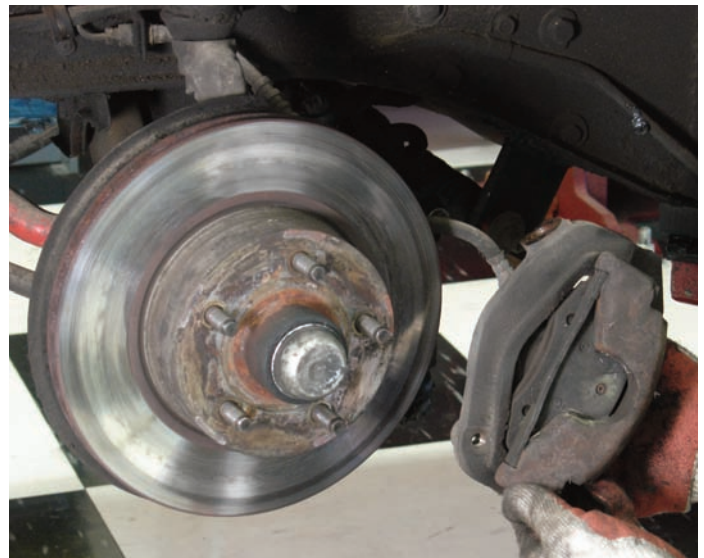
After the caliper bolts were disconnected, the caliper was removed from the car.
