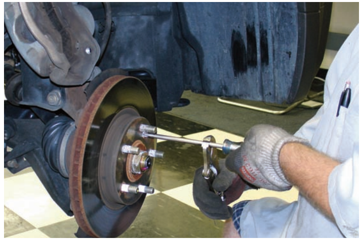
The screws that secure the rotor to the hub were removed with a screwdriver aided by lockjaw pliers. The screws are installed very tight.
