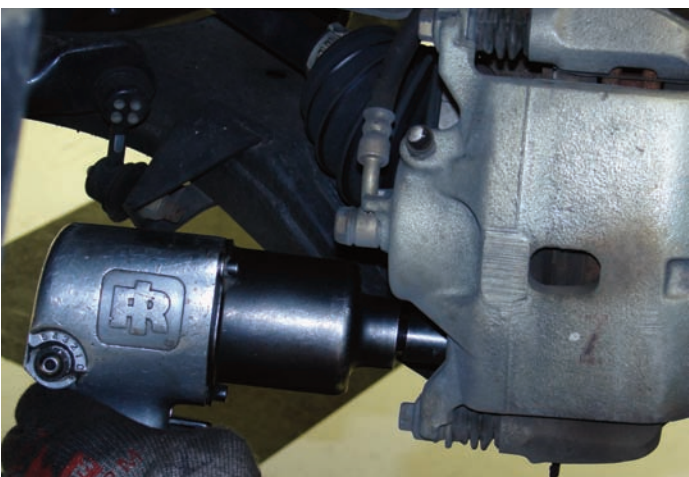
Using an impact gun and the appropriate size socket, the caliper bolts were disconnected and the caliper was removed from the assembly.
