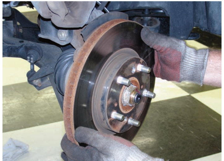
After the mounting screws were disconnected, the rotor was carefully removed from the assembly.
