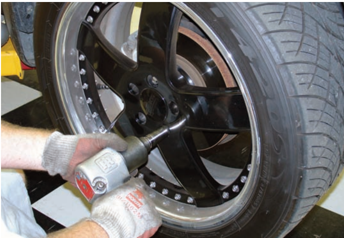
Using an impact gun and the proper size socket, the lug nuts were disconnected, and then the wheels and tires were removed.
