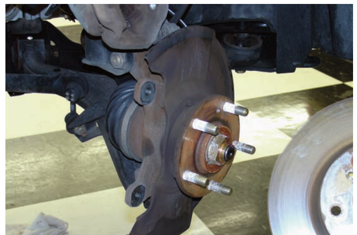
After the rotor disengaged from the centering ring, it was removed and that revealed the hub assembly and the original caliper mounting ears.
