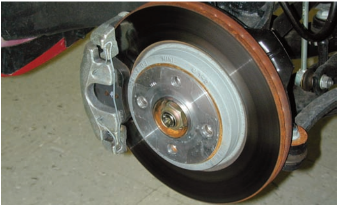
Here is the original brake setup that features heavy cast iron BMW single-piston calipers and rotors.
