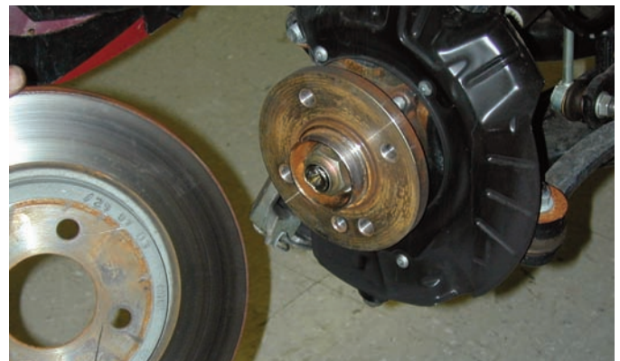
The screw connecting the rotor to the hub assembly was disconnected and then the rotor was removed. Hang on to the screw because it will be reused. With the rotor removed you can see the dust shield that will have to be removed.
