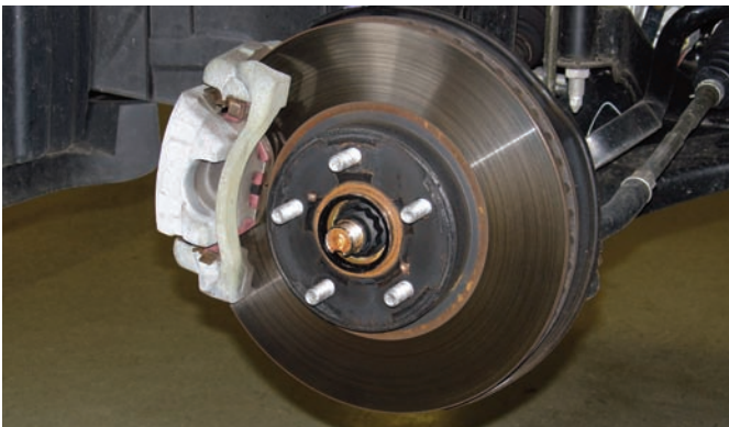
Here is the stock brake system after the wheels and tires were removed. This car uses a single-piston floating caliper for stopping power.
