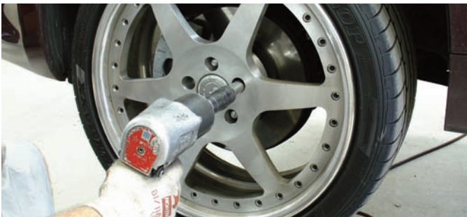
The car was elevated with a floor jack and then jack stands were placed underneath it. Using an impact gun and the appropriate size socket, the lug nuts were disconnected and the wheels and tires were removed.
