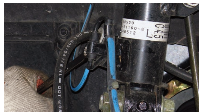
Using a box-end wrench, the bolt securing the built-in hose brake bracket was removed.
