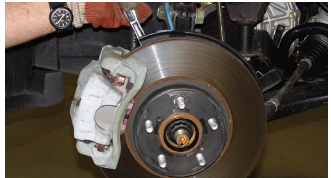
Using a socket wrench and the appropriate size socket, the caliper mounting bolts were disconnected and the caliper was removed, but the hose was not disconnected at this time.
