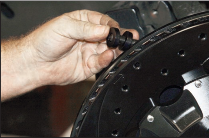
Sequence 14: Lubricate the caliper mounting studs with lightweight oil. Place two spacers on each stud between the bracket and the caliper.
