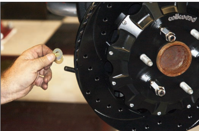
Sequence 15: Initially place two shim washers on each stud between the bracket and caliper.
