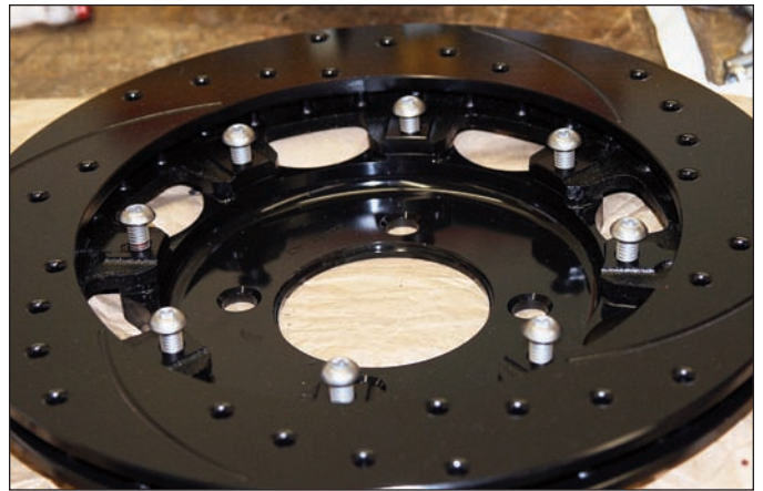
Sequence 10: The hat needs to be bolted to the rotor. Orient the rotor over the hat in the configuration shown above. Apply red Loctite ® 271 to the mounting bolts and thread into the hat.
