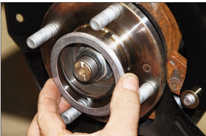
Sequence 9: Install the rotor registration adapter over the axle register against the hub face with the larger O.D. facing inward toward the hub face.
