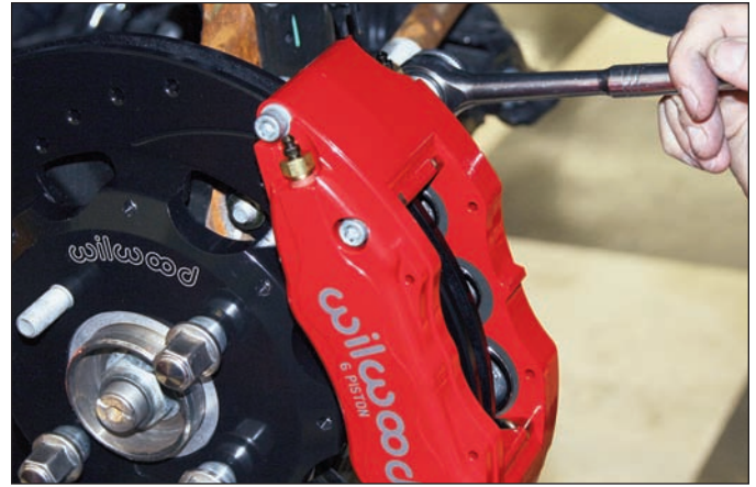
Sequence 16: Mount the caliper onto the bracket so that the largest pistons are at the rotor exit end of the caliper, in relation to the direction of rotor rotation.
