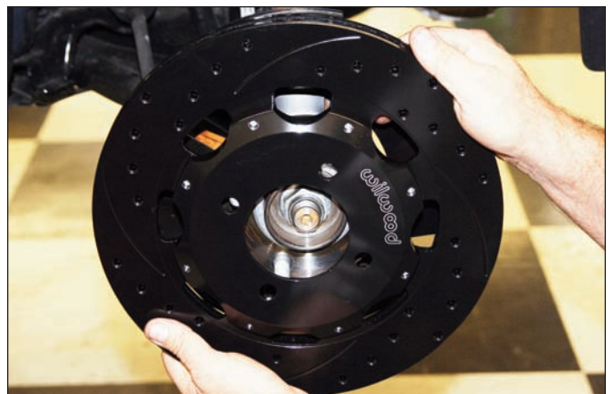
Sequence 12: Install the hat/rotor assembly over the hub assembly. NOTE: The hat/rotor must fit flush against the axle hub flange or excessive rotor run out may result.
