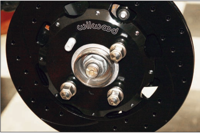
Sequence 13: Secure the hat/rotor with three lug nuts (finger tight) to keep the hat/rotor assembly in place while continuing with the installation.
