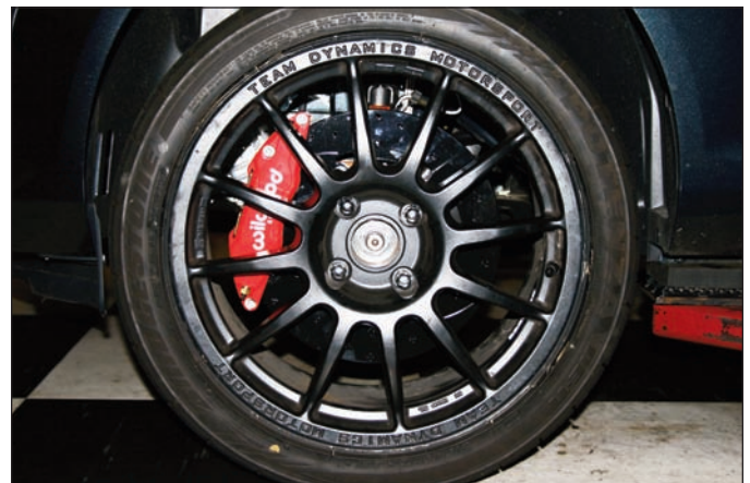
Sequence 23: Install the wheel and torque the lug nuts to manufacturer's specification. Rotate the wheel and check for any interference. Bed in the brake pads and rotor in a safe location before general use driving.
