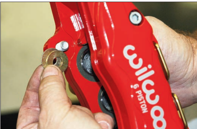
Sequence 15: Initially place two shim washers on each bolt between caliper mounting tab and the mounting ears on the bracket.
