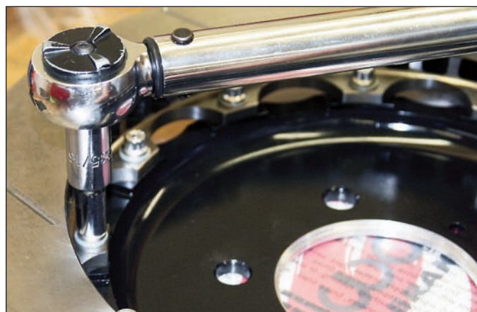
Sequence 17: Place one flat washer over each hole on the rotor mounting tabs. Coat the mounting bolts with red Loctite® 271 and slide through the washer and thread into the hat. Using an alternating sequence, torque bolts to 155 in-lbs.
