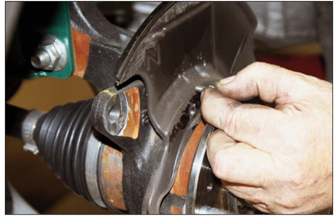
Sequence 10: Remove the screws that secure the dust shield in place.
