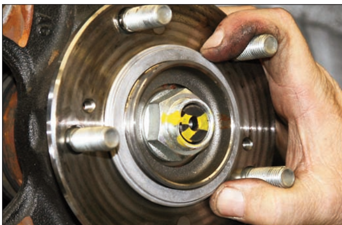
Sequence 15: Install the rotor registration adapter onto the axle register against the hub face with the larger O.D. facing inward toward the hub face.
