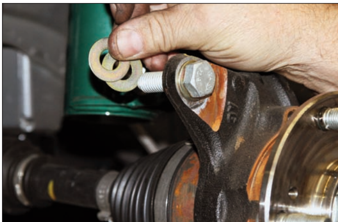
Sequence 13: Initially place one .015" thick shim, and one .033" thick shim between the mounting ear and the caliper mounting bracket.
