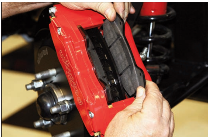
Sequence 19: Insert the brake pads into the caliper with the friction material facing the rotor.
