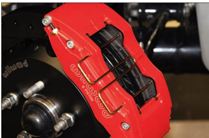
Sequence 20: Secure brake pads in place with the pad clip retainer.
