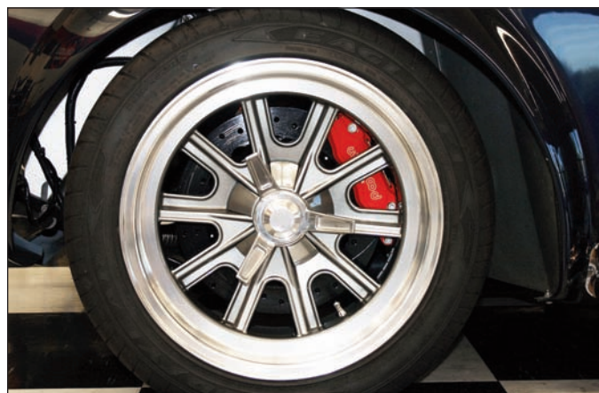
Sequence 22: Install the wheel and torque the lug nuts to manufacturer's specification. Rotate the wheel and check for any interference. Reinstall the replica knock-off's. Bed in the brake pads and rotor in a safe location before general use driving.
